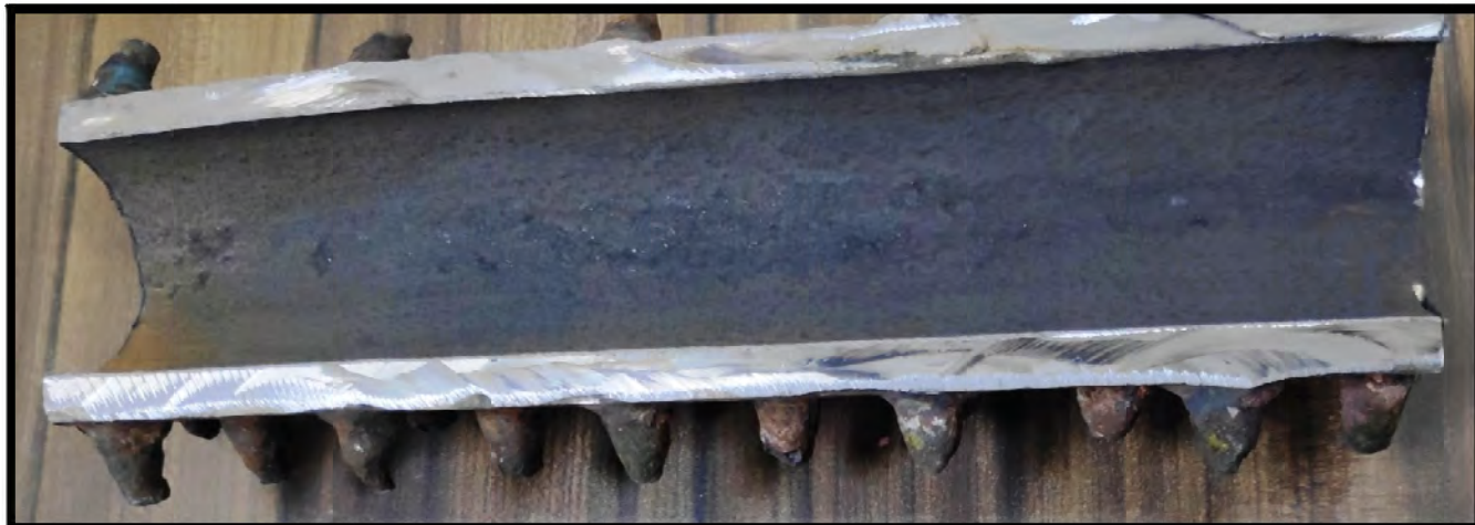
BOTTOM HALF PORTION AFTER CUT IN TWO HALVES, INTERNAL DEPOSITION BY IMPROPER CIRCULATION
