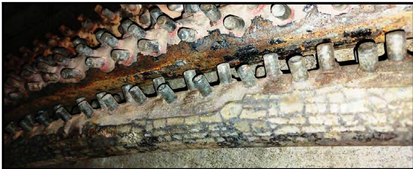
Tube failed location is exactly 12 O'clock position
