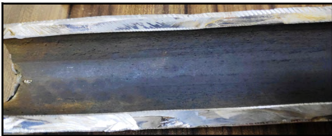
Tube failed location is exactly 12 O'clock position TOP HALF PORTION AFTER CUT IN TWO HALVES, DEEP GROOVE BY FAC & IMPROPER CIRCULATION
